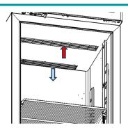
Do not block the equalization valve in SUPERARTIC models
