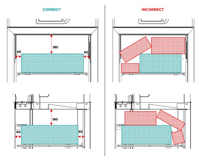
Do not place material in contact with or near the temperature probes.
