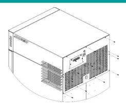
Using a vacuum cleaner or air jet, remove all dust from the condenser fins.
