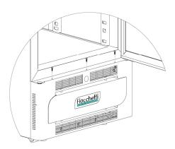
Rotate and pull down the lower panel
