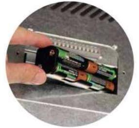
Figure 22 - Batteries tampon
