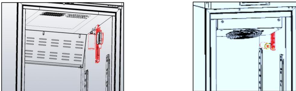
Figure 13– probes position
