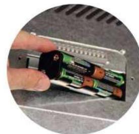
Figure 21 – Buffer batteries
